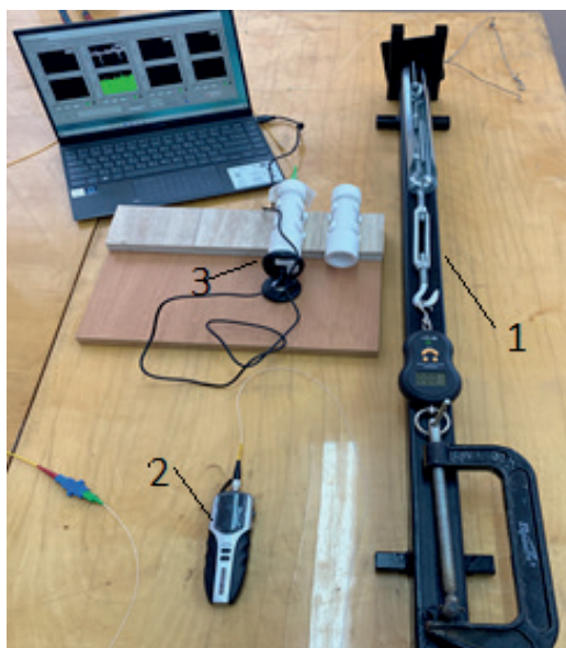
Figure 2 – The laboratory bench of the information-measuring system with the sensor of the roof displacement: 1 – metal frame with elements, 2 – laser radiation source, 3 – web camera
